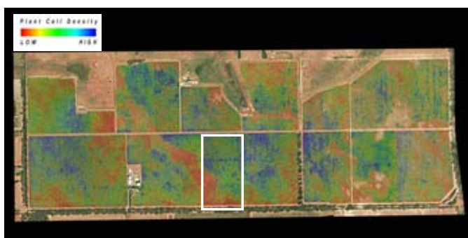
Fig. 1. DMSI data shown as a plant cell density (PCD) image grading from low PCD (red), through to medium PCD (green), to high PCD (dark blue). The Cabernet Sauvignon block (delineated by the white rectangle) was used to ground-truth the imagery and was later harvested differentially.
